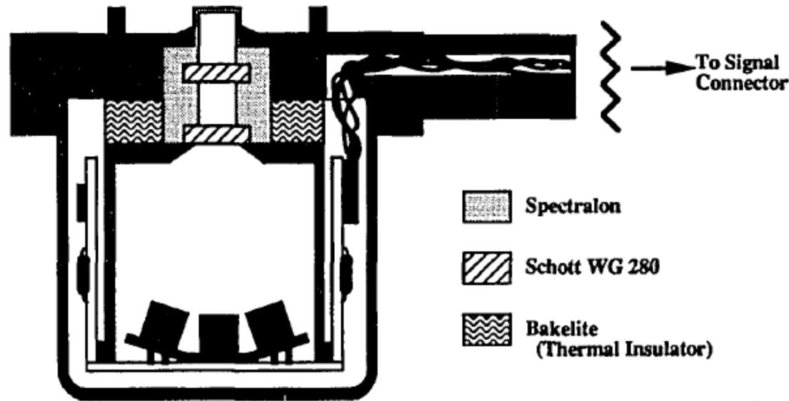
Fig. 2. Multifilter detector cross section (not to scale).
