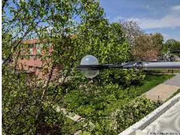
**On the right** : installation at Millersville University, PA for measurement of net solar irradiance (difference between downwelling and upwelling solar irradiance)
