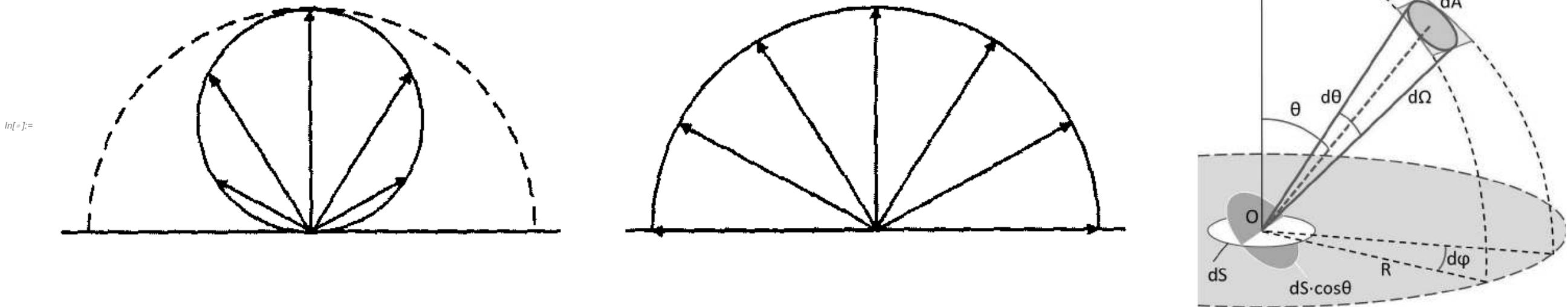
Note the difference between Total Horizontal Irradiance and Actinic Flux. **On the left** : Horizontal Irradiance is related to a horizontal detection area. Photons are weighted with the cosine of their angle of incidence. This is why a low sun provides less heat to the Earth's surface than a high sun. **In the center** : Actinic flux density, for instance, as seen by an ozone
