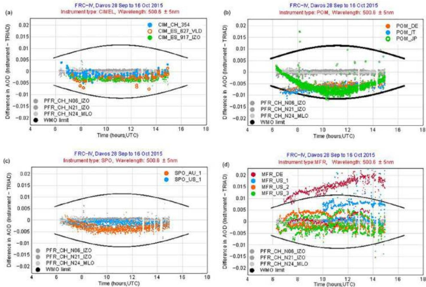
**Figure 2.** Comparison of the triad (gray points) with the Cimel instruments (a,  $500 \pm 5$  nm), POM instruments (b,  $500 \pm 5$  nm), SPO instruments (c,  $500 \pm 5$  nm) and with the MFR instruments (d,  $862 \pm 5$  nm). Different colors represent different instruments for all the five comparison days, and gray lines represent the WMO AOD limits.
