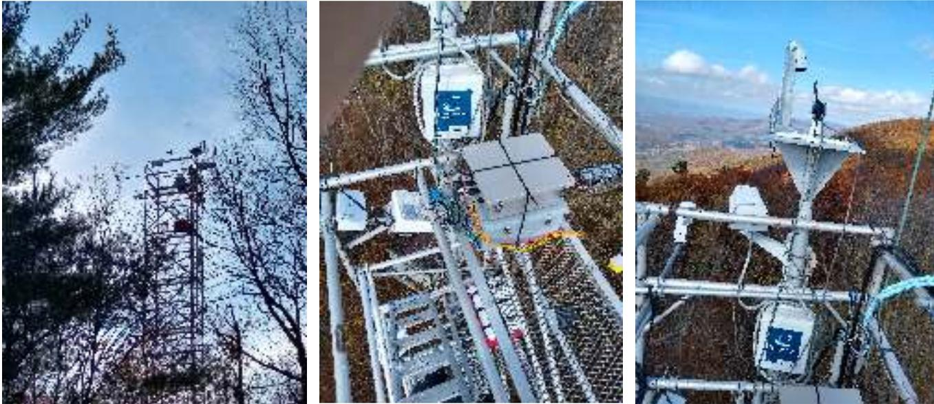
To calculate  $\text{Ln}[V_0]$  from MFRSR data acquired at the Pinnacles tower in the Shenendoah mountains.
