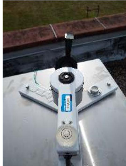
Then UMBC undergrad and NCAS - M student, Wambugu Kironji, works on the interface boxes for the MFRSRs being set up on the roof of the main building at HU Beltsville. The setup requires high accuracy in pointing (toward geographic south), leveling, timing. When operating the rotating band alternatively shadows in three positions as shown.
